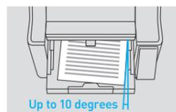
The tilt of the document is controlled by rollers on both sides.
